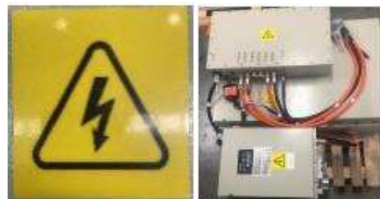
Figure 8.7.1 Warning Signs and Orange High Voltage Connection Lines
