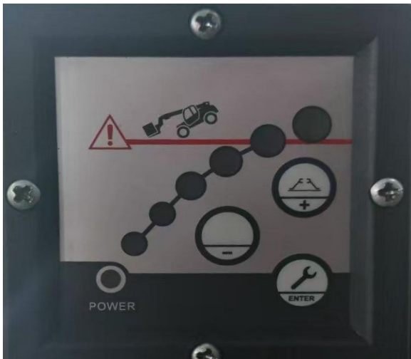
Figure 3.2.20-1 Longitudinal Stability Limiting Device (SAR)
